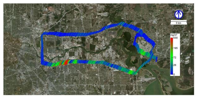
Figure 13 HSC SOF alkane measurement, 26 September, 11:39 - 13:03. Marker size and color scale proportional to slant column in mg/m<sup>2</sup>. Note color scale is logarithmic so smaller plumes are visible. Line from the marker points upwind in the direction of the source with length proportional to wind speed.
