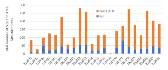
Figure 1 Number of Site and Area direct emission measurements per day. Total number of measurements depends on sky and wind conditions and area of focus. More measurements are made on days in areas with a greater number of distinguishable sources, e.g. Lynchburg Ferry & La Porte. QAQC criteria include parameters like wind speed, cloud interference, source interference, instrument performance.
