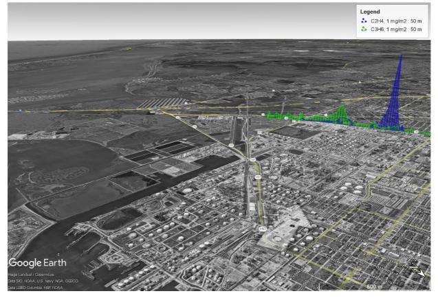
Figure 19. SOF ethylene (blue) and propylene (green) measurement at Texas City, 8 September, about 2:10 AM. The apparent height of the overlay is proportional to the ethylene and propylene column, respectively. Wind direction (Northeast) during the measurement is indicated with a white arrow. Image mapped on Google Earth © 2022.
