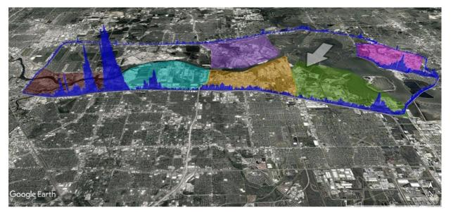
Figure 31 SOF Alkane measurement showing temporary or upset emissions from an unknown source in the west of the HSC, 26 September, approximately 12:30 PM when the dominant plumes were passed. The apparent height of the blue overlay is proportional to the alkane column. Wind direction (NE) during the measurement is shown with a white arrow. Image mapped on Google Earth © 2022.
