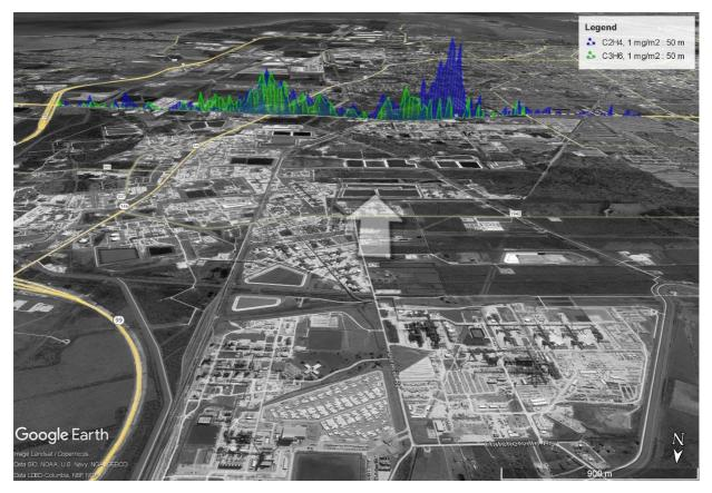
Figure 17. SOF ethylene (blue) and propylene (green) measurement at Mont Belvieu, 21 September, about 09:15 AM. The apparent height of the overlay is proportional to the ethylene and propylene column, respectively. Wind direction (North) during the measurement is indicated with a white arrow. Image mapped on Google Earth © 2022.
