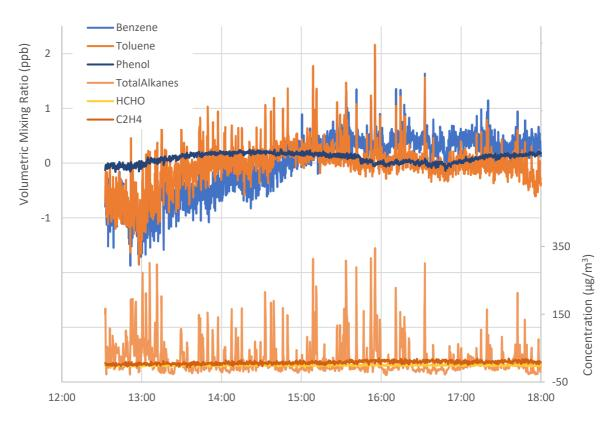
Figure 29 Example of time-series data during intercomparison for a few selected compounds. Benzene, toluene and phenol volumetric mixing ratios from the MEDOAS instrument are shown on the upper left axis and alkanes, formaldehyde and ethylene concentrations from MEFTIR are shown on the lower right axis.
