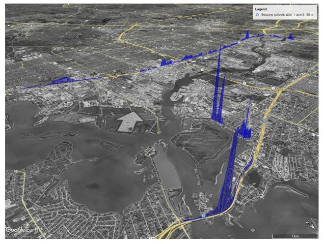
Figure 24. Example of concentration mapping data from MeDOAS showing benzene (blue) in the HSC area. Winds from the northeast as indicated by the white arrow. Composite of several measurements from the 12, 23 and 26 September. Image mapped on Google Earth © 2022.
