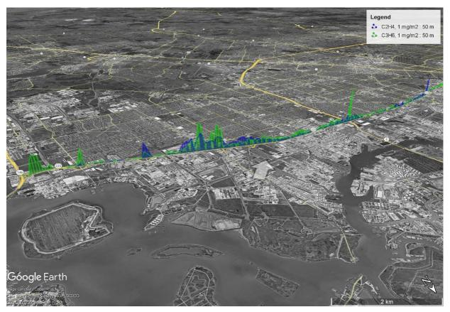
Figure 10. SOF ethylene (blue) and propylene (green) measurement at HSC, 27 September, about 11:00 AM. The apparent height of the overlay is proportional to the ethylene and propylene column, respectively. Wind direction (NE ~5 m/s) during the measurement is indicated with a white arrow. Image mapped on Google Earth © 2022.
