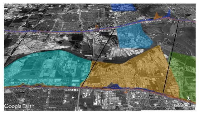
Figure 30 Example of concentration mapping data from MeDOAS showing benzene (blue, max 20 ppb) and Toluene (orange, max 18 ppb), in the Deer Park & Pasadena area and north of HSC, 09:39 - 17:57, 26 September. Winds from the east-northeast. Image mapped on Google Earth © 2022.
