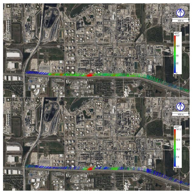
Figure 26 Extractive measurements of alkane (top) and BTEX (bottom) concentrations of the Deer Park area. Color scale and marker size proportional to concentration and line points upwind in direction of the source. Note: Color scale is logarithmic.
