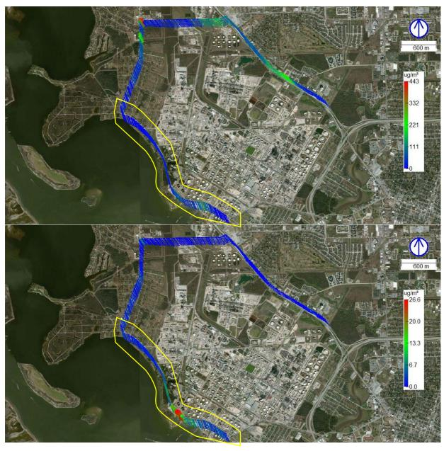
Figure 23 Extractive measurements of alkane (top) and benzene (bottom) concentrations at Baytown Facility fenceline. Color scale and marker size proportional to concentration and line points upwind in direction of the source. Yellow ringed area exluded from total facility indirect flux measurements with southerly winds. The mass ratio of BTEX/alkanes for the source in the port is about 0.5.
