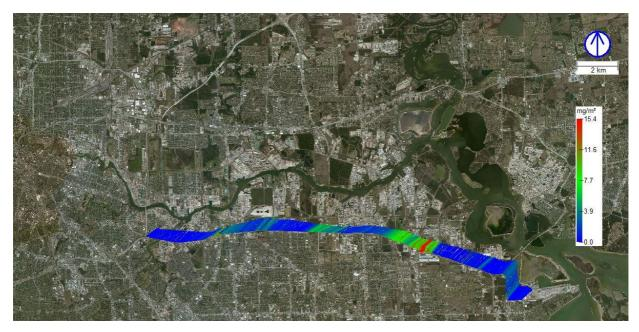
Figure 11 HSC SOF ethylene measurement, 27 September, 10:53 - 11:16. Marker size and color scale proportional to slant column in mg/m<sup>2</sup>. Note color scale is logarithmic so smaller plumes are visible. Line from the marker points upwind in the direction of the source with length proportional to wind speed.
