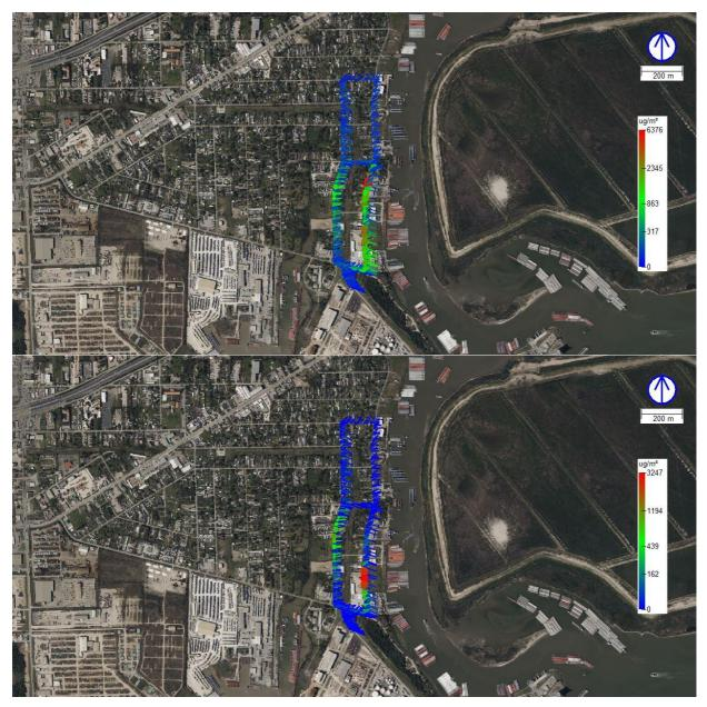
Figure 25 Extractive measurements of alkane (top) and benzene (bottom) concentrations in the Channelview area. Color scale and marker size proportional to concentration and line points upwind in direction of the source. Note: Color scale is logarithmic.
