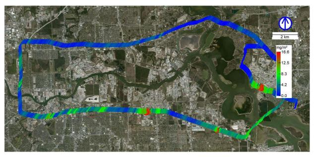
Figure 21 HSC SkyDOAS NO<sub>2</sub> measurement, 26 September, 11:39 - 13:03. Marker size and color scale proportional to vertical column in mg/m<sup>2</sup>. Line from the marker points upwind in the direction of the source with length proportional to wind speed.
