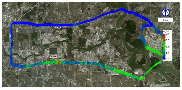
Figure 20 HSC SkyDOAS HCHO measurement, 26 September, 11:39 - 13:03. Marker size and color scale proportional to vertical column in mg/m<sup>2</sup>. Line from the marker points upwind in the direction of the source with length proportional to wind speed.
