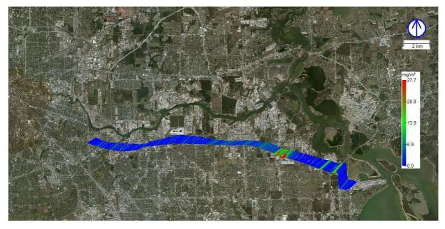
Figure 12 HSC SOF propylene measurement, 27 September, 10:53 - 11:16. Marker size and color scale proportional to slant column in mg/m<sup>2</sup>. Line from the marker points upwind in the direction of the source with length proportional to wind speed.
