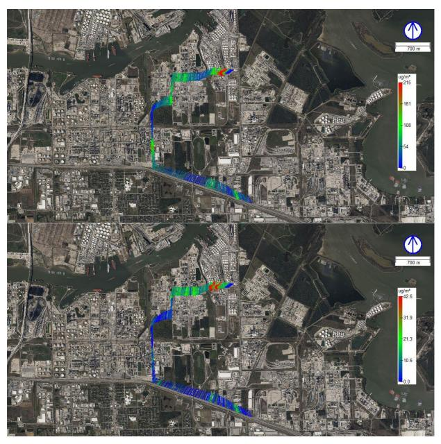
Figure 27 Extractive measurements of alkane (top) and BTEX (bottom) concentrations of the Tidal Road area. Color scale and marker size proportional to concentration and line points upwind in direction of the source.
