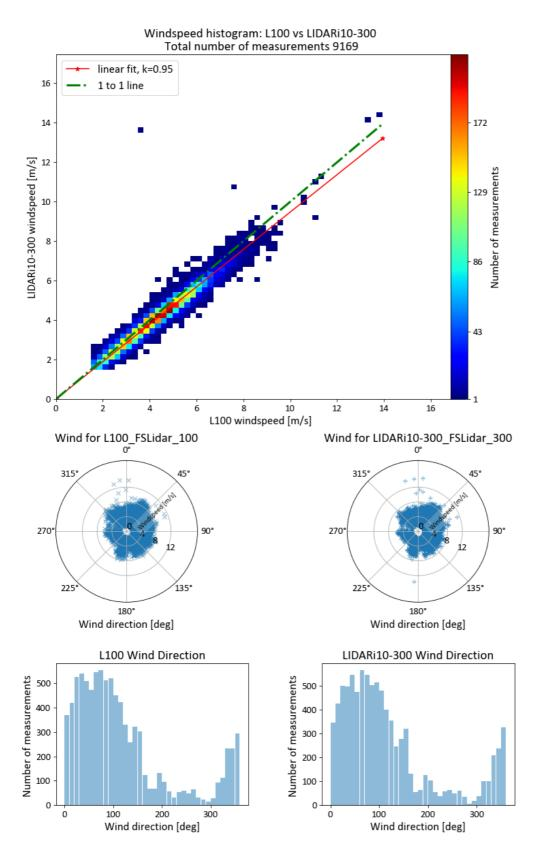
Figure 2 Example of wind speed data collected during the survey comparing the integrated 10 - 300 m (LIDARi10-300) winds to the 100 m (L100) measurement.
